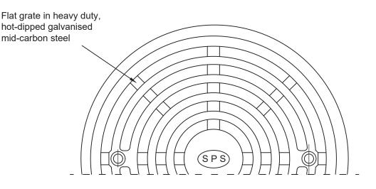
Load-tested to Class D of AS3996-2006
