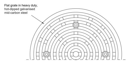
Load-tested to class D of AS3996-2006
