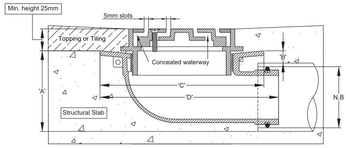
Spigot pushes into 65mm PVC or copper with o-ring connection, or connects to 50mm PVC/HDPE with no-hub coupling.
