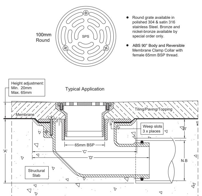
Outlet pushes into 65mm PVC or copper with o-ring connection, or connects to 50mm PVC/HDPE with no-hub coupling.
