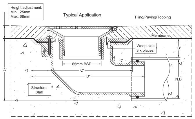
Outlet pushes into 65mm PVC or copper with o-ring connection, or connects to 50mm PVC/HDPE with no-hub coupling.
