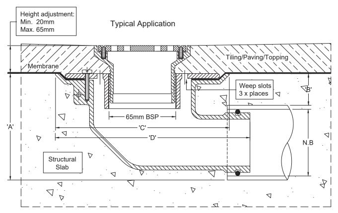
Outlet pushes into 65mm PVC or copper with o-ring connection, or connects to 50mm PVC/HDPE with no-hub coupling.
