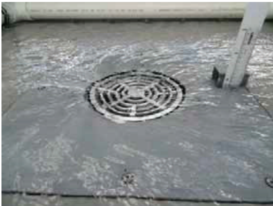
Weir Flow 8 L/s (30mm)
