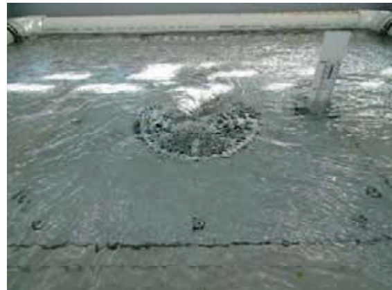
Surcharged flow 12 L/s (90mm)
