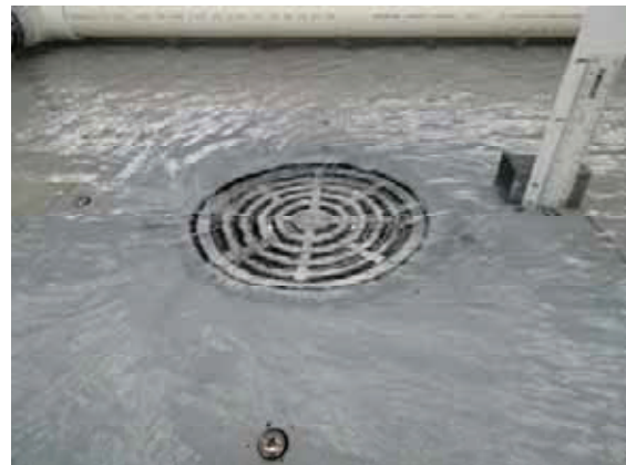
Vortex/surcharged flow 4 L/s (20mm)
