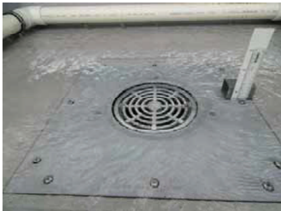
Weir Flow – 3 L/s (13mm)
