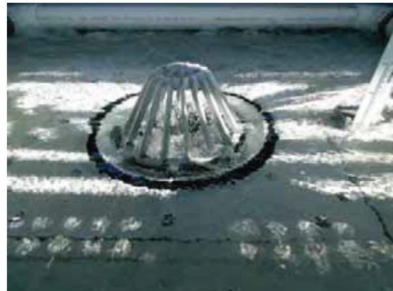
Surcharged Flow - 20 L/s (40mm)
