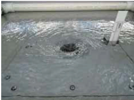
Weir Flow – 2.5 L/s (50mm)
