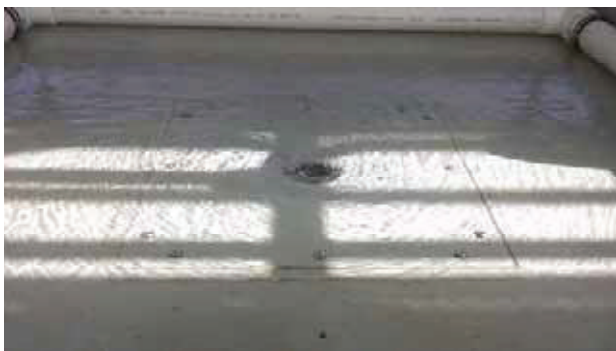
Weir flow – 1 L/s (50mm)
