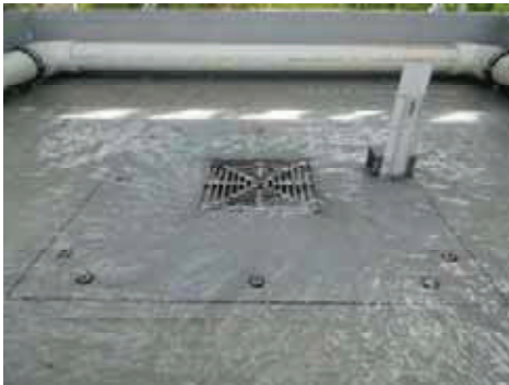
Weir Flow – 2.0 L/s (20mm)
