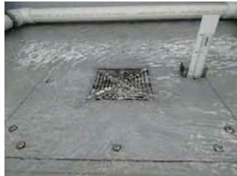
Orifice flow – 4.0 L/s (30mm)
