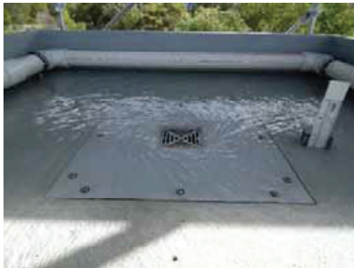
Weir flow - 1 L/s (20mm)
